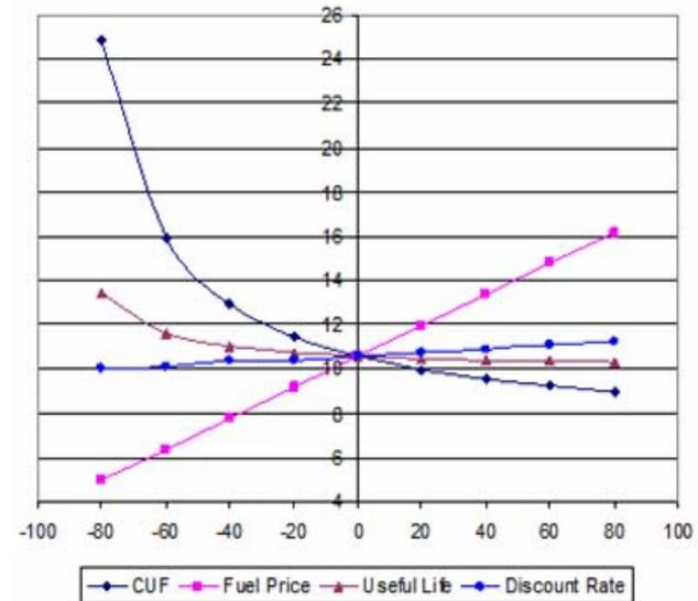
Figure 4. Sensitivity analysis of cost of generation through SVO genset
