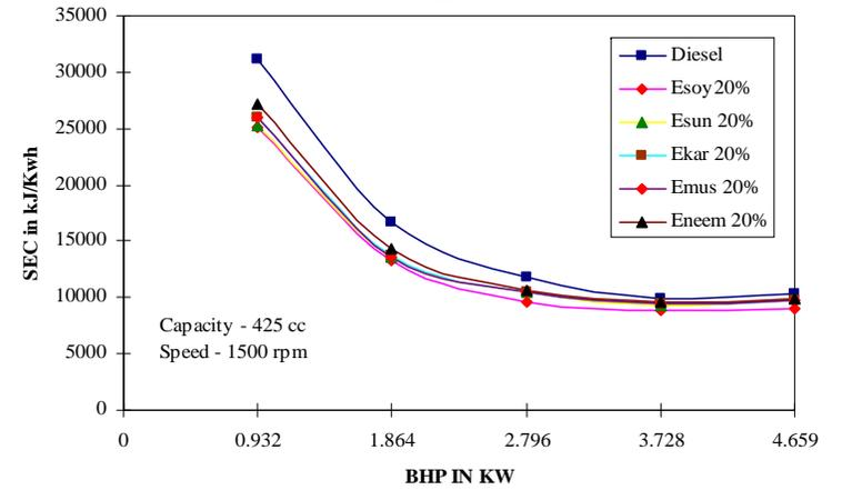
Figure 5: Variations in SFC with Respect to BHP for 20% by Volume Blends of Five Different Vegetable Oils
