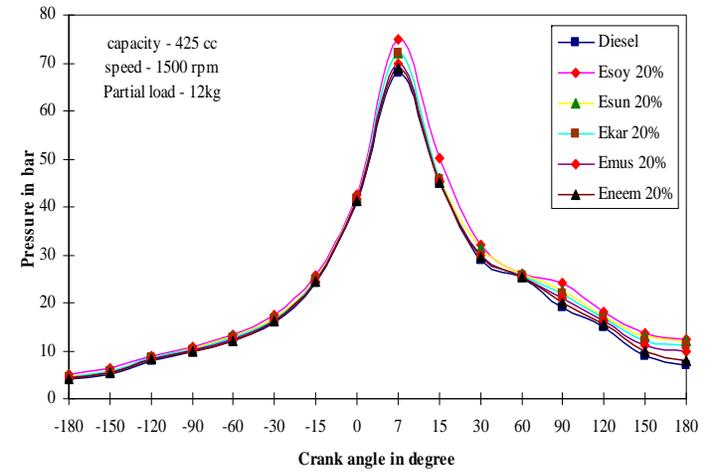
Figure 7(c): Variations in CPP at Full Load with Respect to Crank Angle for 20% by Volume Blends of Five Different Vegetable Oils
