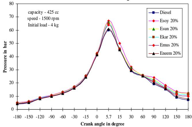
Figure 7(b): Variations in CPP at Partial Load with Respect to Crank Angle 20% by Volume Blends of Five Different Vegetable Oils.
